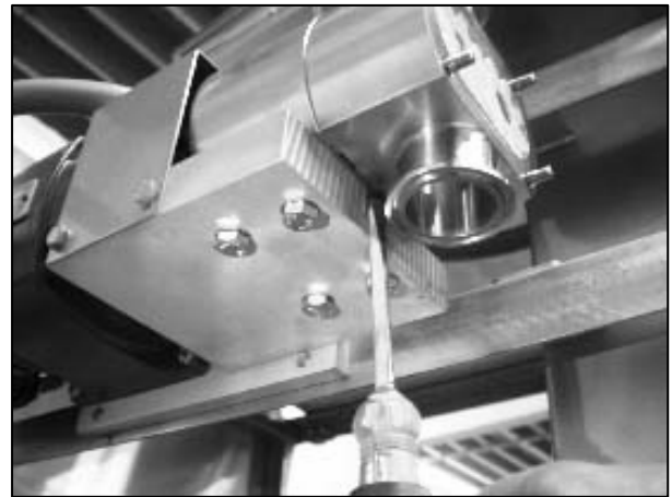
38. Insert a flat tip screw driver into the slot to loosen the pump body if it can not be removed by hand.
